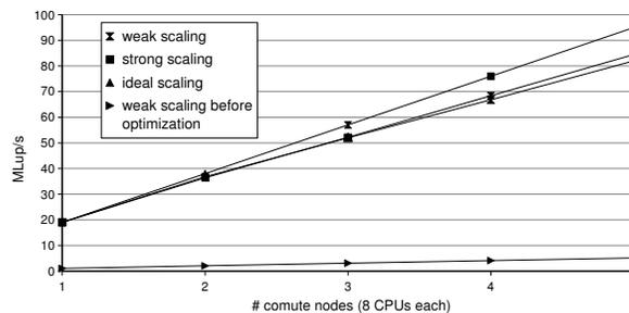
Figure 2: Offline simulations without steering and visualization: The application shows good performance measured in MLup/s (million lattice site updates per second) and high efficiency for strong and weak scaling with 86 and 89 %, respectively. Additionally, the plot visualizes the striking improvement in performance as compared to the non-optimized version of the code.
