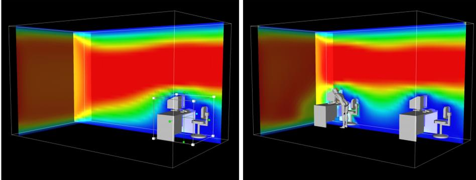
Figure 6: Snapshots of air-flow configurations for two different furniture scenarios of an office room in an interactive case study.
