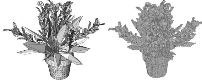
Figure 1: Discretization of a CAD-generated geometry: On the left a plant object's approximation using 30014 triangles is shown facing its discrete representation (30074 voxel, grid resolution 100x100x100) on the right. The voxelization takes only 0.19 seconds on an AMD Dual Opteron with 2.4 GHz.
