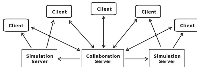
Figure 4: Overview of the multidisciplinary collaboration platform. Clients may contact different servers, or no simulation server at all; however, they need to have access to a collaboration server to report changes or be notified about changes to the application set-up which may have been initiated by other users. The collaboration server, of course, has to forward incoming modification signals to the simulation.
